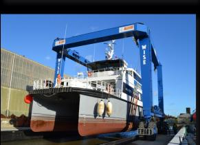
One of the UK's largest and most capable boat lift. The 200T provides a fast and secure lift for vessels up to 200 tonnes, 40m in length and 11m beam. Four independently controlled wheels and multi-mode steering enable precise manoeuvrability around the facility. The lift has a built in digital weighing system to enable the safe positioning of the vessel in the hoist. An ideal lift for boat repairs, inspection, or hull defouling to improve performance. A faster and safer alternative to
